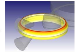
This 'state of the art' system utilizes an ALE solver with automated time stepping. The model uses brick (8 node) elements and supports fully automatic adaptive
