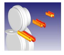
Lagrangian solver is available to study the transient effects throughout the process, while an ALE option predicts the 'steady state' behavior.
