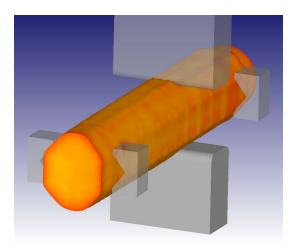
bite size and the time between bites and passes. A simulation preview is provided to identify potential input errors prior to FEM calculations. This enables the user to run cogging simulations without user intervention.
