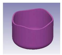
Hill's anisotropy model captures these directional effects. In addition to the normal flow stress curve, it requires only the data from three tension test samples cut at specific directions relative to the rolled sheet.
